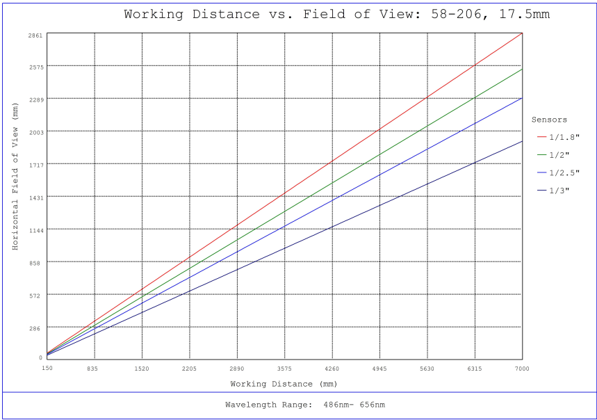
#58-206, 17.5mm FL f/2.5, Blue Series M12 Lens, Working Distance versus Field of View Plot
