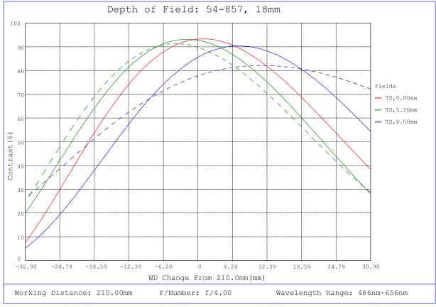
#54-857, 18mm DG Series Fixed Focal Length Lens, Depth of Field Plot, 210mm Working Distance, f4
