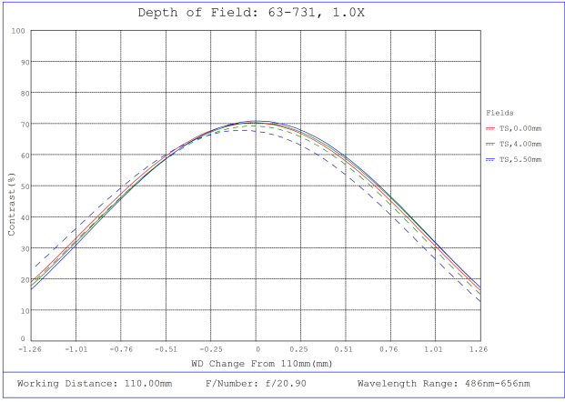
#63-731, 1X, 110mm WD CompactTL™ Telecentric Lens, Depth of Field Plot, 110mm Working Distance, f20.9
