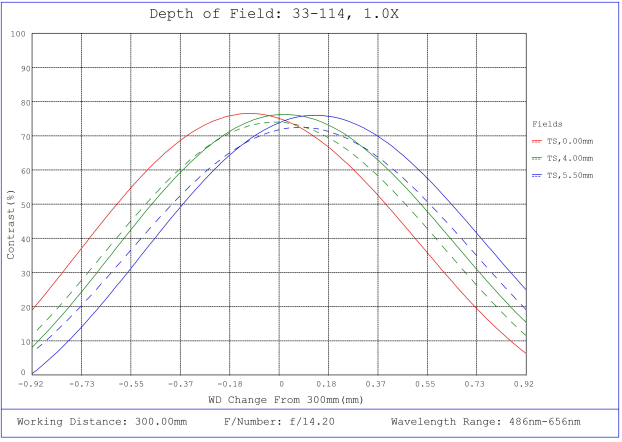
#33-114, 1X, 300mm WD, In-Line CompactTL™ Telecentric Lens, Depth of Field Plot, 300mm Working Distance, f14.2
