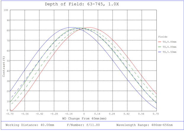
#63-745, 1X, 40mm WD CompactTL™ Telecentric Lens, Depth of Field Plot, 40mm Working Distance, f11
