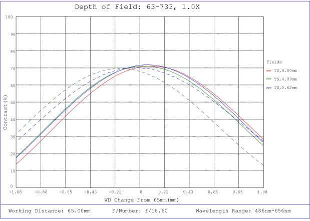
#63-733, 1X, 65mm WD CompactTL™ Telecentric Lens, Depth of Field Plot, 65mm Working Distance, f18.6
