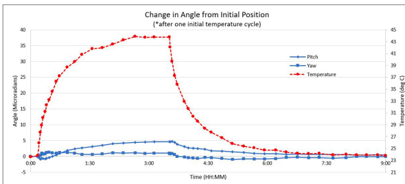
Performance of the Ultraprecision Gimbal Mirror Mount When Exposed to a 20°C Temperature Change
