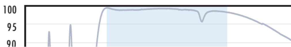
Fused Silica with NIR II Coating Typical Transmission
