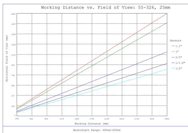
#55-326, 25mm DG Series Fixed Focal Length Lens, Working Distance versus Field of View Plot
