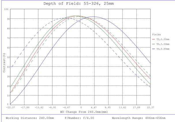
#55-326, 25mm DG Series Fixed Focal Length Lens, Depth of Field Plot, 240mm Working Distance, f4
