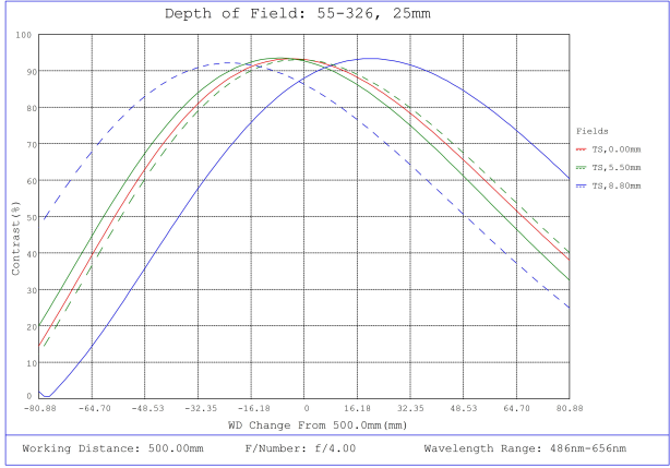
#55-326, 25mm DG Series Fixed Focal Length Lens, Depth of Field Plot, 500mm Working Distance, f4
