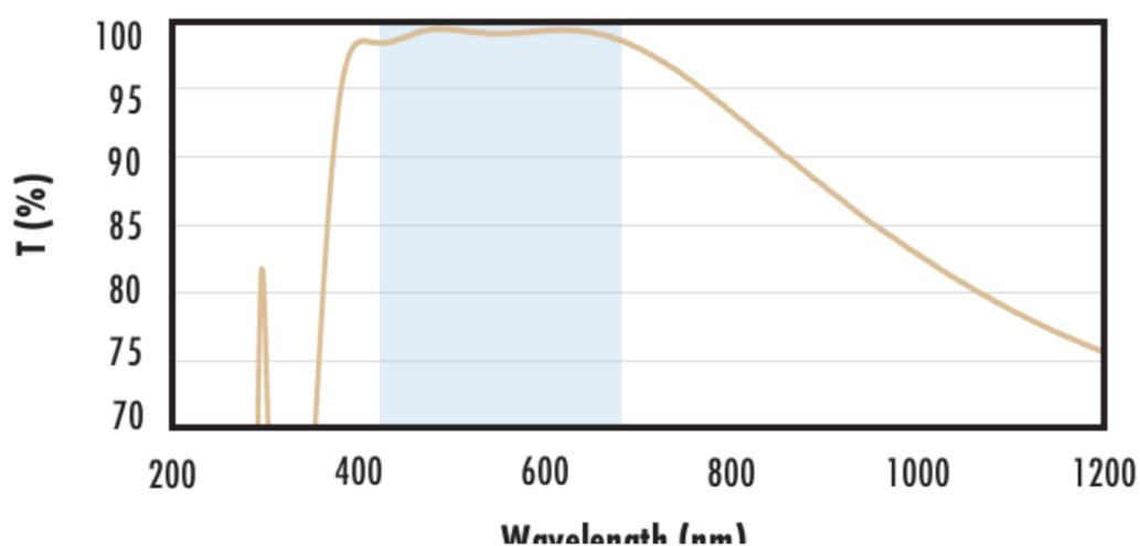
Typical transmission of a 3mm thick fused silica window with VIS 0° (425-675nm) coating at 0° AOI.
