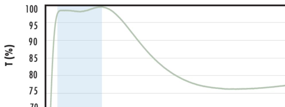
Typical transmission of a 3mm thick fused silica window with UV-AR (250-425nm) coating at 0° AOI.
