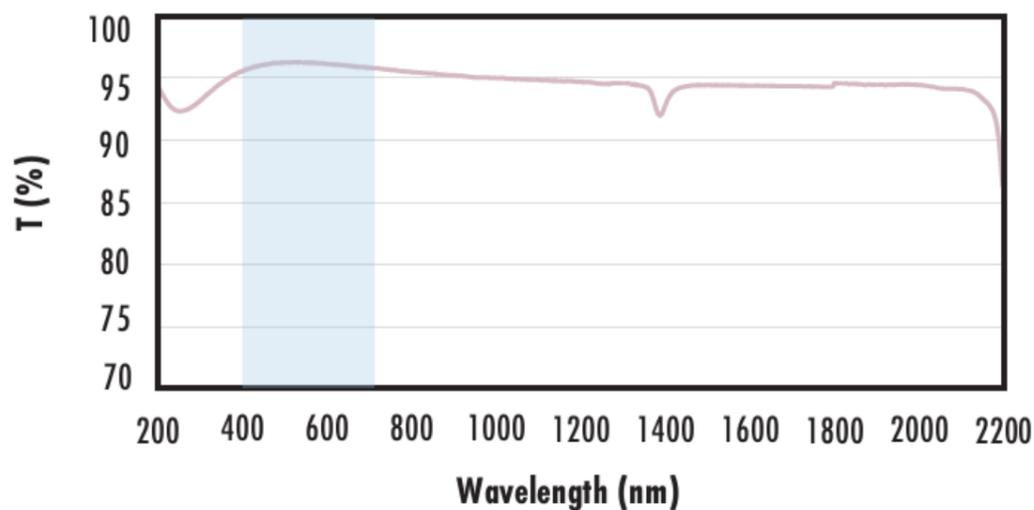
Typical transmission of a 3mm thick fused silica window with MgF<sub>2</sub> (400-700nm) coating at 0° AOI.
