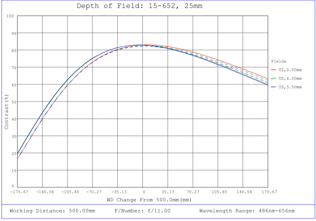
#15-652, 25mm, f/11 Cw Series Fixed Focal Length Lens, Depth of Field Plot, 500mm Working Distance, f11
