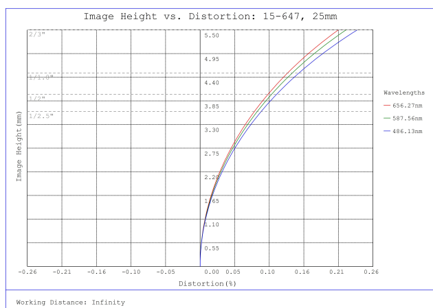
#15-647, 25mm, f/1.8 Cw Series Fixed Focal Length Lens, Distortion Plot
