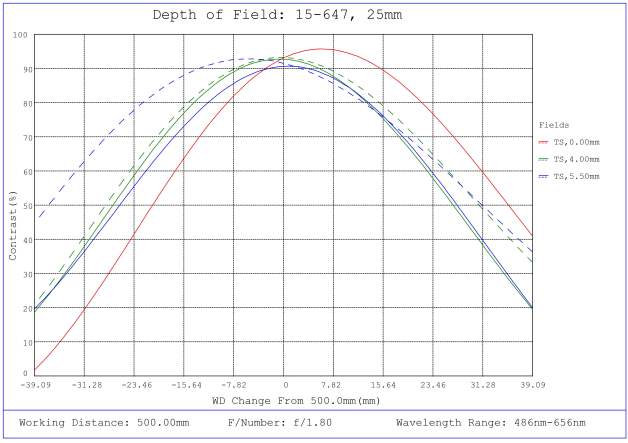
#15-647, 25mm, f/1.8 Cw Series Fixed Focal Length Lens, Depth of Field Plot, 500mm Working Distance, f1.8
