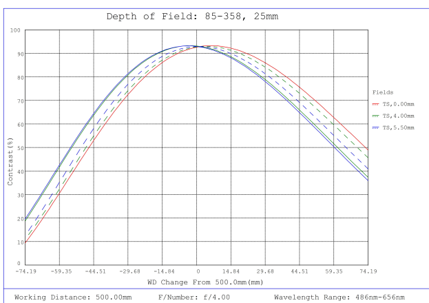
#85-358, 25mm, f/4 Ci Series Fixed Focal Length Lens, Depth of Field Plot, 500mm Working Distance, f4
