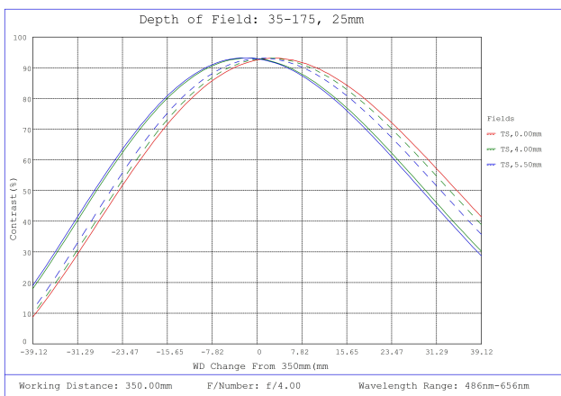
#35-175, 25mm, f/4 Cr Series Fixed Focal Length Lens, Depth of Field Plot, 350mm Working Distance, f4
