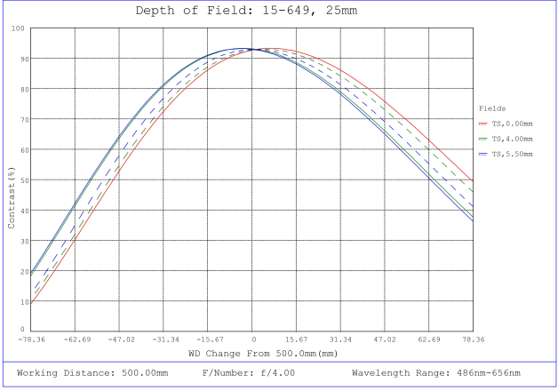
#15-649, 25mm, f/4 Cw Series Fixed Focal Length Lens, Depth of Field Plot, 500mm Working Distance, f4
