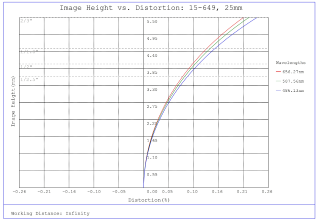
#15-649, 25mm, f/4 Cw Series Fixed Focal Length Lens, Distortion Plot
