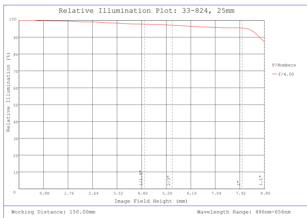
#33-824, 25mm f/4.0, HPI Series Fixed Focal Length Lens, Relative Illumination Plot
