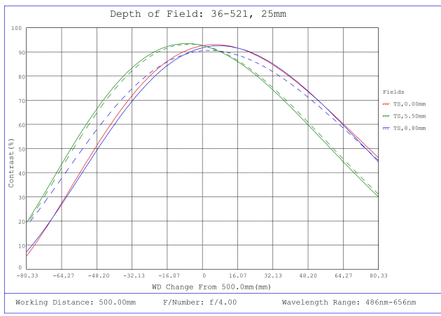
#36-521, 25mm f/4.0, HPr Series Fixed Focal Length Lens, Depth of Field Plot, 500mm Working Distance, f4
