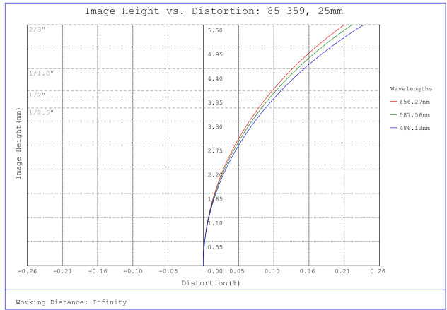
#85-359, 25mm, f/5.6 Ci Series Fixed Focal Length Lens, Distortion Plot
