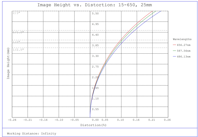
#15-650, 25mm, f/5.6 Cw Series Fixed Focal Length Lens, Distortion Plot
