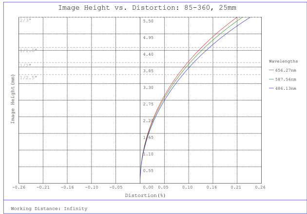
#85-360, 25mm, f/8 Ci Series Fixed Focal Length Lens, Distortion Plot
