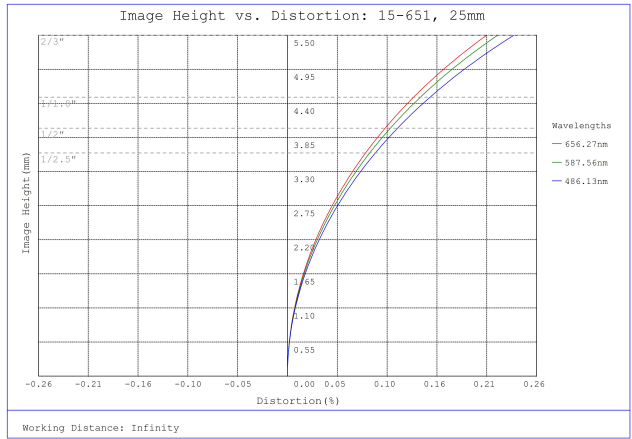
#15-651, 25mm, f/8 Cw Series Fixed Focal Length Lens, Distortion Plot
