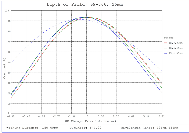
#69-266, 25mm FL f/4, Blue Series M12 Lens, Depth of Field Plot, 150mm Working Distance, f4
