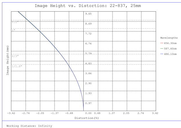
#22-837 - 25mm Focal Length, UAV Series Fixed Focal Length Lens, Distortion Plot
