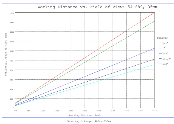
#54-689, 35mm DG Series Fixed Focal Length Lens, Working Distance versus Field of View Plot
