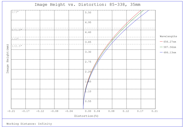
#85-338, 35mm, f/16 Ci Series Fixed Focal Length Lens, Distortion Plot
