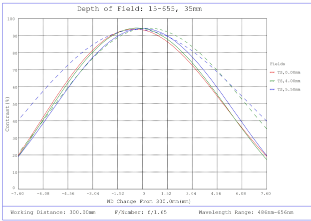
#15-655, 35mm, f/1.8 Cw Series Fixed Focal Length Lens, Depth of Field Plot, 300mm Working Distance, f1.6
