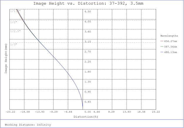
#37-392, 3.5mm, f/2 Cr Series Fixed Focal Length Lens, Distortion Plot
