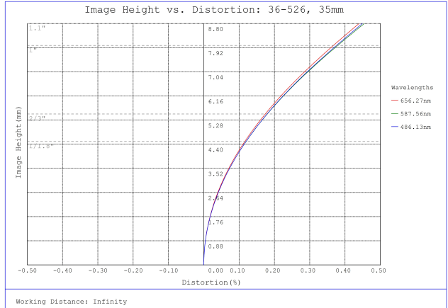
#36-526, 35mm f/2.0, HPr Series Fixed Focal Length Lens, Distortion Plot
