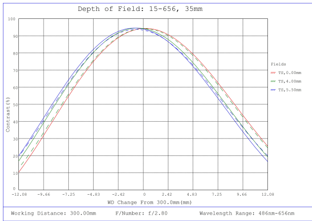
#15-656, 35mm, f/2.8 Cw Series Fixed Focal Length Lens, Depth of Field Plot, 300mm Working Distance, f2.8
