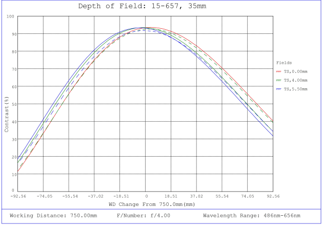
#15-657, 35mm, f/4 Cw Series Fixed Focal Length Lens, Depth of Field Plot, 750mm Working Distance, f4
