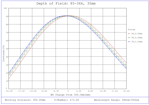
#85-366, 35mm, f/5.6 Ci Series Fixed Focal Length Lens, Depth of Field Plot, 300mm Working Distance, f5.6
