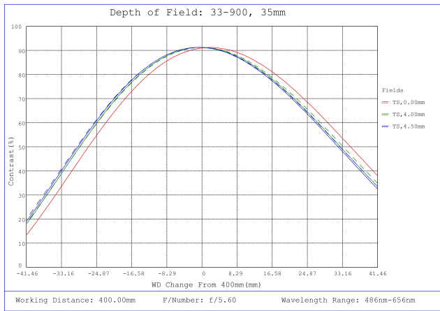
#33-900, 35mm f/5.6, UCi Series Fixed Focal Length Lens, Depth of Field Plot, 400mm Working Distance, f5.6
