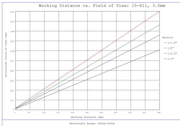
#15-611, 3.5mm f/8.0 Sealed Cw Series Fixed Focal Length Lens, Working Distance versus Field of View Plot
