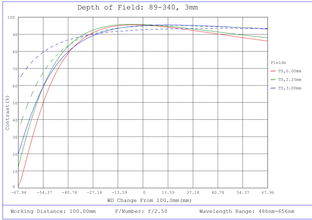
#89-340, 3mm FL f/2.5, Blue Series M12 Lens, Depth of Field Plot, 100mm Working Distance, f2.5
