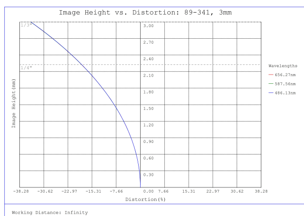
#89-341, 3mm FL f/4.0, Blue Series M12 Lens, Distortion Plot
