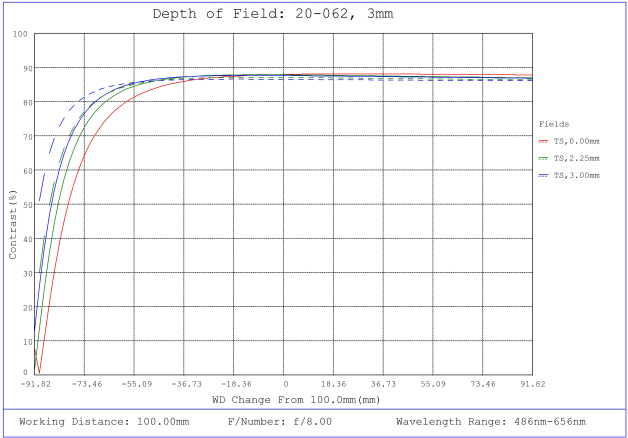
#20-062, 3mm FL f/8.0 IR-Cut Rugged Blue Series M12 Lens, Depth of Field Plot, 100mm Working Distance, f8
