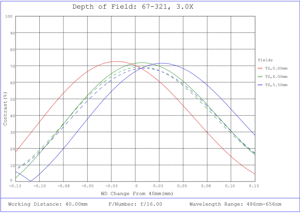
#67-321, 3X, 40mm WD, In-Line CompactTL™ Telecentric Lens, Depth of Field Plot, 40mm Working Distance, f16
