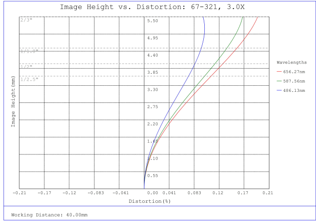
#67-321, 3X, 40mm WD, In-Line CompactTL™ Telecentric Lens, Distortion Plot
