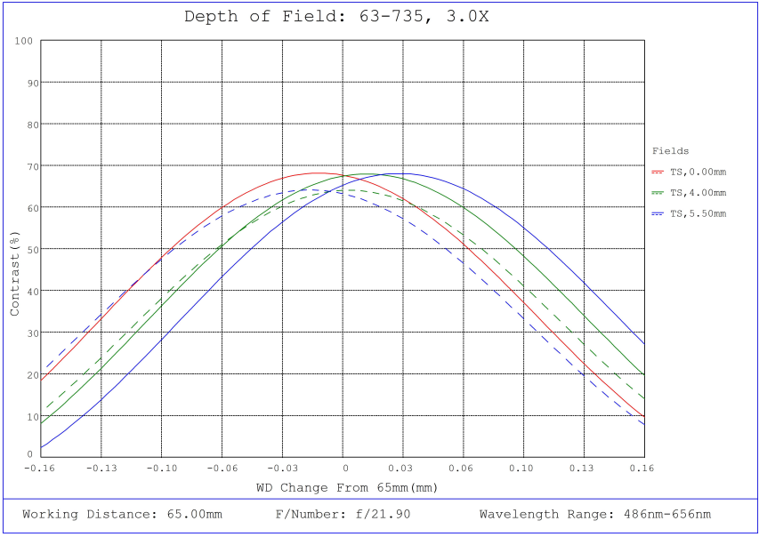
#63-735, 3X, 65mm WD CompactTL™ Telecentric Lens, Depth of Field Plot, 65mm Working Distance, f21.9
