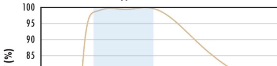
Typical transmission of a 3mm thick N-BK7 window with VIS 0° (425-675nm) coating at 0° AOI.
