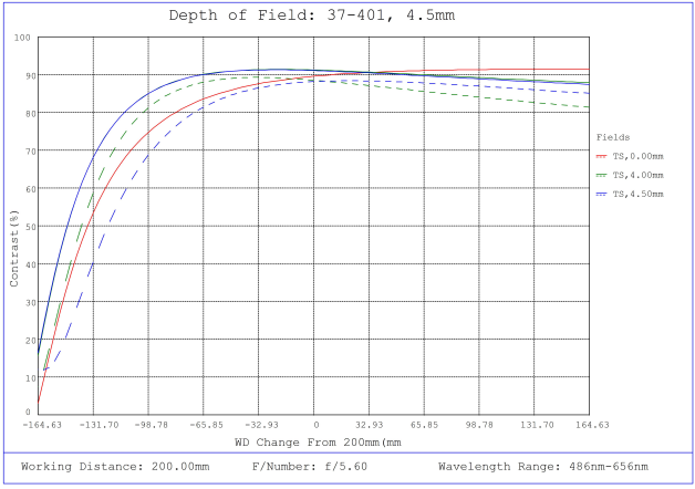
#37-401, 4.5mm, f/5.6 Cr Series Fixed Focal Length Lens, Depth of Field Plot, 200mm Working Distance, f5.6
