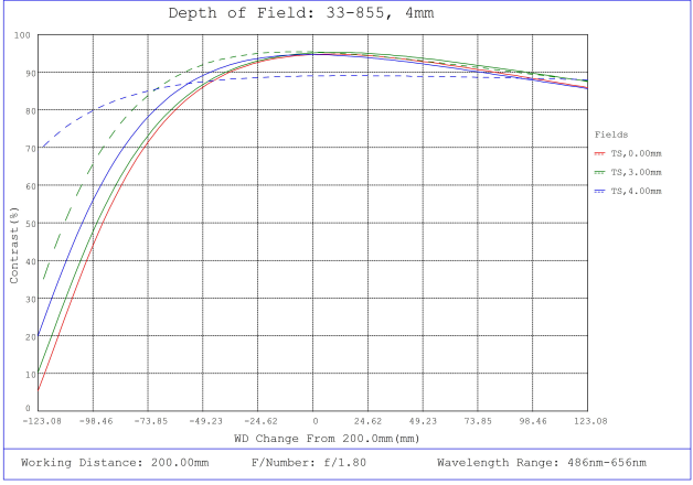
#33-855, 4mm, f/1.8 UCi Series Fixed Focal Length Lens, Depth of Field Plot, 200mm Working Distance, f1.8
