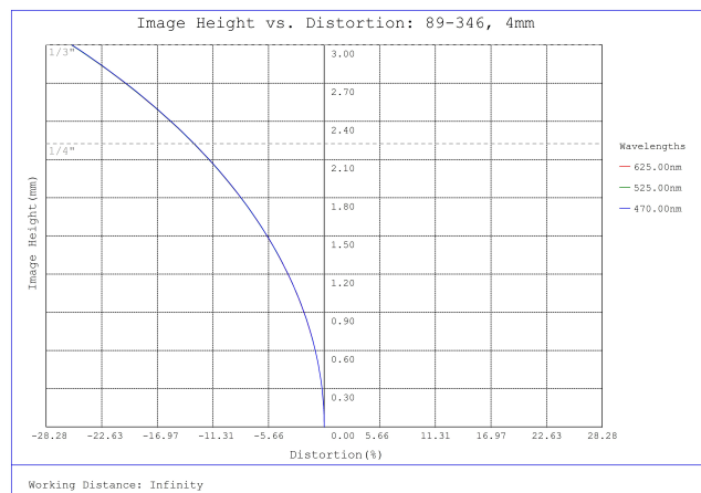
#89-346, 4mm FL f/5.6, Blue Series M12 Lens, Distortion Plot
