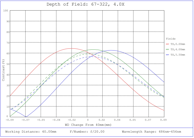
#67-322, 4X, 40mm WD, In-Line CompactTL™ Telecentric Lens, Depth of Field Plot, 40mm Working Distance, f20
