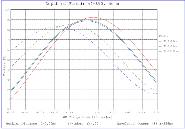
#54-690, 50mm DG Series Fixed Focal Length Lens, Depth of Field Plot, 240mm Working Distance, f4
