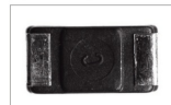
It's difficult to make an image of the electrode part using a Bar Light.
