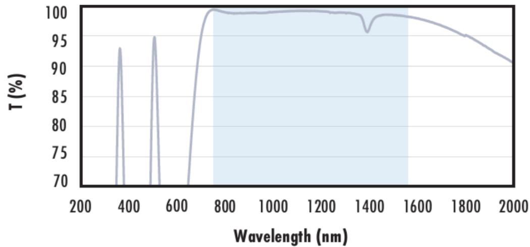
Typical transmission of a 3mm thick fused silica window with NIR II (750 - 1550nm) coating at 0° AOI.
