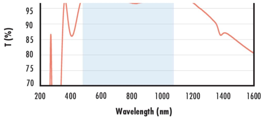
Typical transmission of a 3mm thick fused silica window with YAG-BBAR (500-1100nm) coating at 0° AOI.
