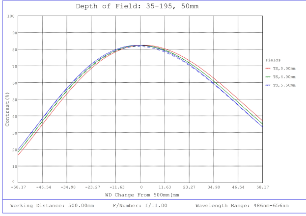
#35-195, 50mm, f/11 Cr Series Fixed Focal Length Lens, Depth of Field Plot, 500mm Working Distance, f11
