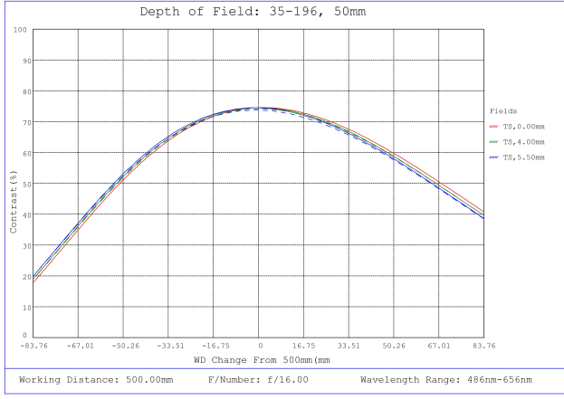
#35-196, 50mm, f/16 Cr Series Fixed Focal Length Lens, Depth of Field Plot, 500mm Working Distance, f16
